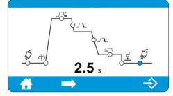
**Miller 4TS trigger functionality** – Gives access to hot start or cold start from the torch trigger
