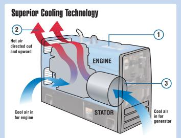
Directed airflow improves cooling for long engine and component life.
